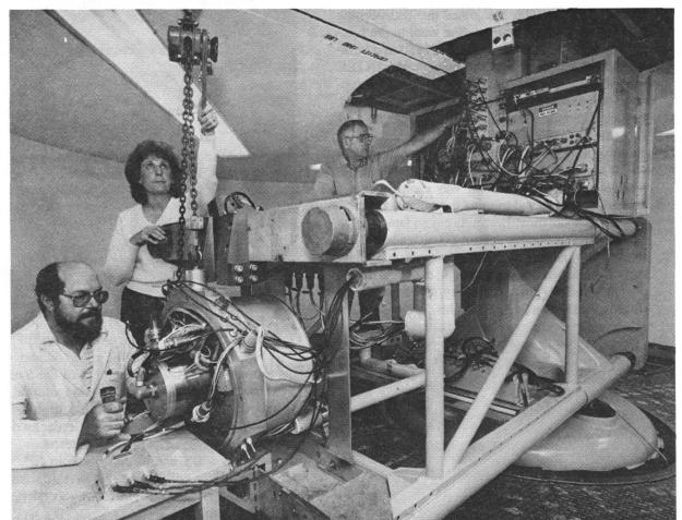
AN EIGHT-FOOT-LONG CENTRIFUGE — one of two in the 7264 test lab — goes from creep to full speed (270 rpm) in 300 milliseconds; the fast-rise capability duplicates gravity (g) forces that a weapon might experience during in-flight maneuvers. Here, Fred Trussell (left), Marilyn Higley, and Chuck Collier mount a W87 test assembly on the centrifuge before a test. The machine, used to test 23 different weapon systems, subjects test items to g loads of up to 50,000 pounds.
